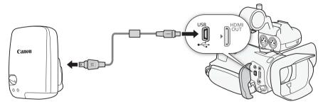
When connecting the GP-E2 GPS Receiver to the camcorder, use the connecting cable supplied with the receiver.
