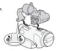
2 Firmly tighten the front and rear screws with a coin or similar object.
