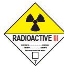
Category III-YELLOW Does not exceed 2 mSv/h at any location on the external surface of the package and the transport index does not exceed 10.
