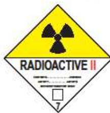
Category II-YELLOW Does not exceed 500 µSv/h at any location on the external surface of the package and the transport index does not exceed 1.
