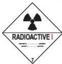
Category I-WHITE Does not exceed 5 µSv/h at any location on the external surface of the package
